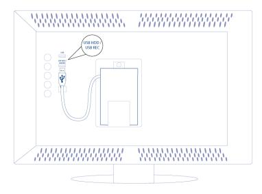
**Cable management:** If necessary, you can wind the cable around the clip.
