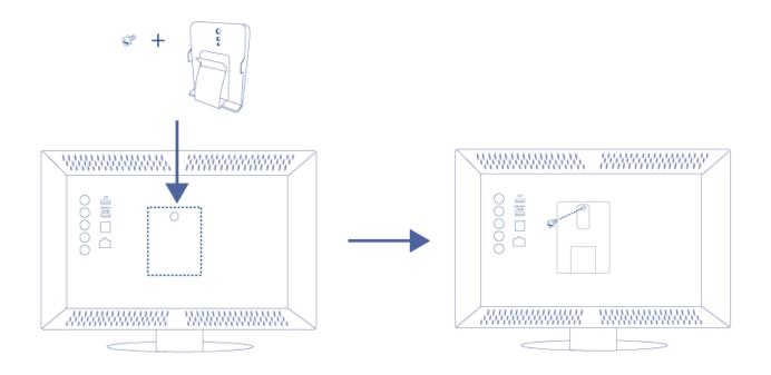
Once the mounting kit is properly installed, slide the RikikiTV into the clip.
