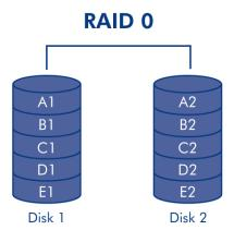
BIG (also called RAID 0 or "Spanning" in some LaCie devices), allows for the fastest data transmission and capacity of the different RAID settings. Requiring at least 2 drives, RAID 0 stripes data onto each disk. The available capacities of each disk are added together so that one logical volume mounts on the computer.
