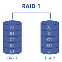
SAFE mode (also referred to as RAID 1) is a secure RAID mode that requires at least 2 drives and works with pairs of drives. One logical volume mounts on the computer and the combined available capacity of both drives is limited to the capacity of the lowest-capacity disk. If one physical disk fails, the data is available immediately on the second disk. No data is lost if one disk fails.
