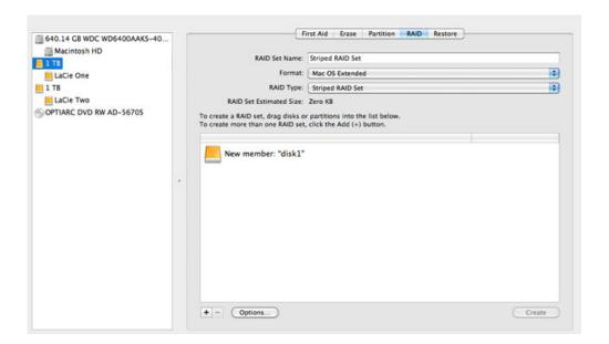
12. Drag the second drive to the same field in the middle of the RAID tab.
