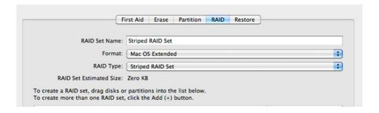
11. Drag one of the drives to the empty field in the middle of the RAID tab.
