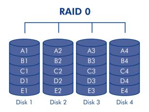
**Caution:** In a RAID 0 array, if one physical drive in the array fails, the data of all drives becomes inaccessible because parts of the data have been written to all drives.
