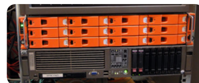
Reynaertcollege runs VMware for enhanced network management. To make certain that critical operations are never interrupted, VMware's proprietary VMDK files are stored on the LaCie 12big Rack Fibre arrays.
