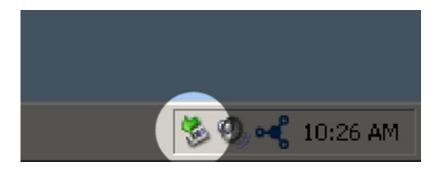
This message will appear: "Safe to Remove Hardware" (or similar). It is now safe to disconnect the device.
